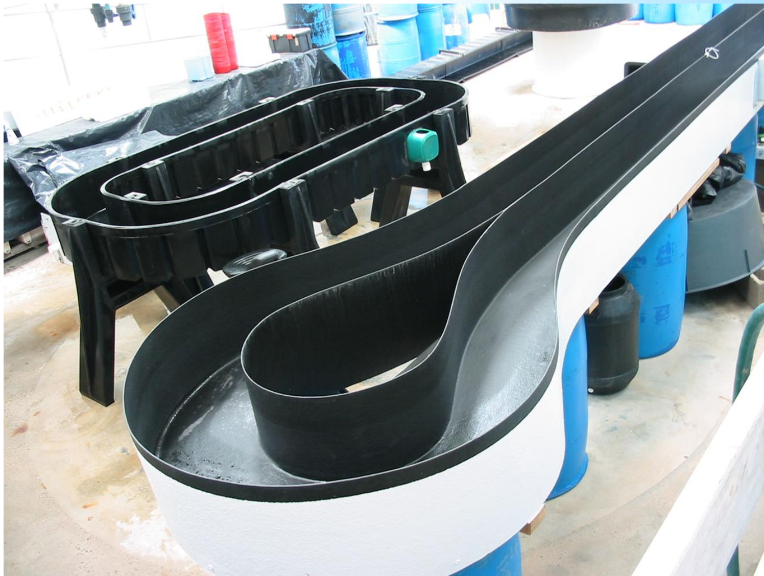
Comparison between 300mm width raceway and 300m width “Dog-bone” raceway
