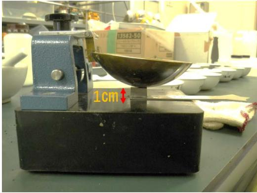
Fig 4-4 落下高調整
