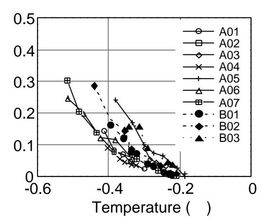
Fig 18. Relationship between growth rate of the warmest ice lens and temperature at the growth surface.
