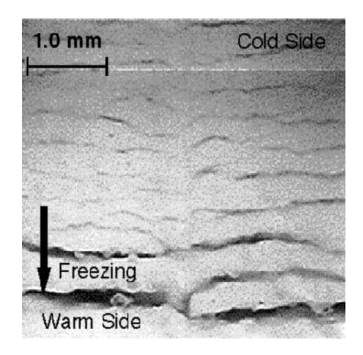
Fig. 20c. An image of the freezing sample 5s (water saturated non-uniform size glass particles) under the conditions of A2 ( $V_s = 0.6 \, \mu m/sec$ ,  $= 0.20 \, ^{\circ}C/mm$ ).
