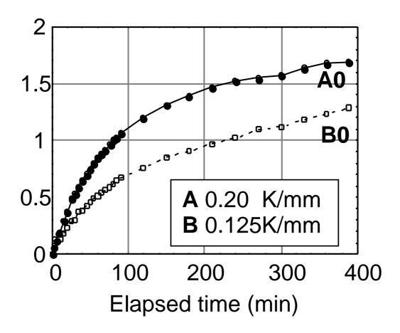
Fig. 16a. The change in thickness of the warmest ice lens in the sample 1 for specimens A0 and B0.
