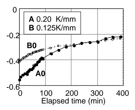
Fig. 17a. Temperatures at the growth surface of the warmest ice lens observed in sample 1.
