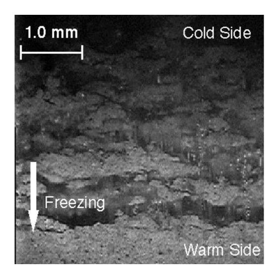
Fig. 20a. An image of the freezing sample 1 (Fujinomori soil) under the condition of A2 ( $V_s = 0.6 \ \mu m/sec$ , = 0.20 °C/mm).
