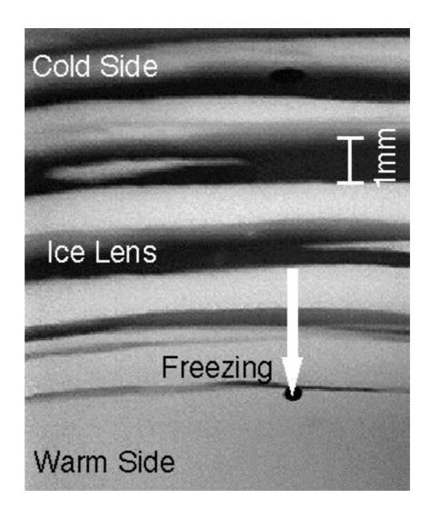
Fig. 20b. An image of the freezing sample 4 (glass particles) under the condition of D2 ( $V_s = 0.8 \ \mu m/sec$ , = 0.20 °C/mm).
