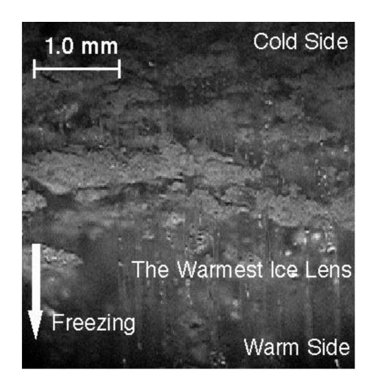
Fig. 15a. An image of the freezing sample 1 (Fujinomori soil) under the condition of A0 ( $V_s = 0 \ \mu m/sec$ , = 0.20 °C/mm).
