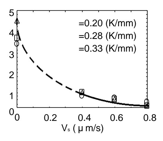
Fig. 21. Relationship between freezing rate and thickness of ice lens.
