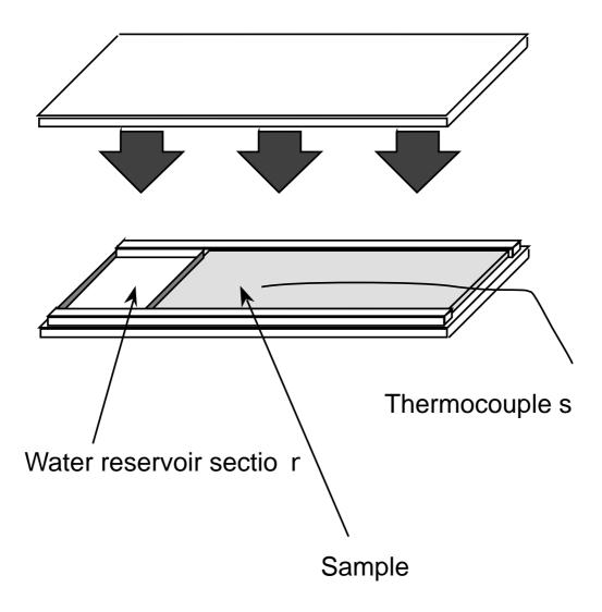
Fig. 14. Schematic diagram of sample cell for unidirectional freezing experiment.
