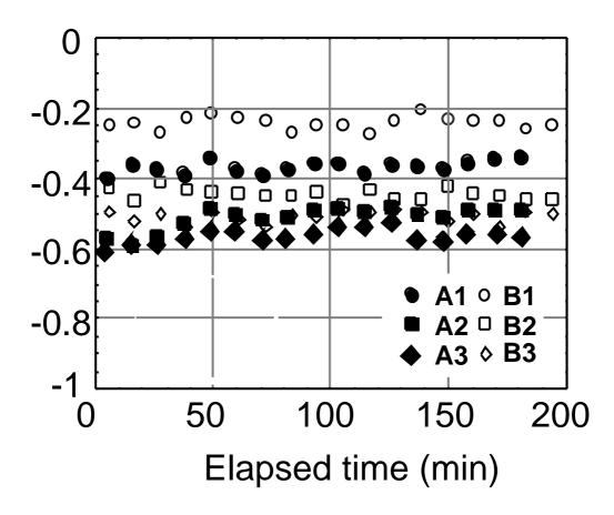
Fig. 25. Temperature at growth surface of ice lenses.
