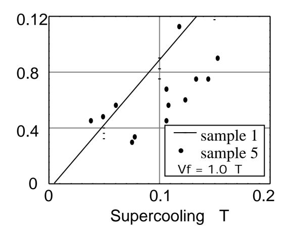
Fig. 19. Relationship between the growth rate of ice lens and supercooling degree at the growth surface.
