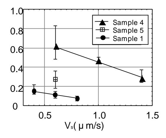
Fig. 22. Relationship between freezing rate and spacing between ice lenses.
