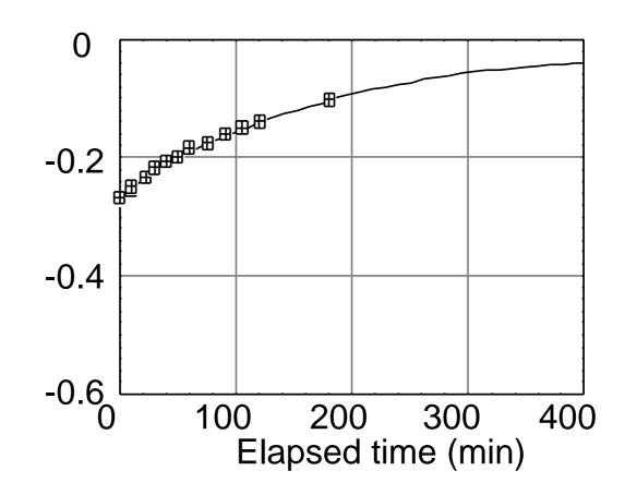
Fig. 17b. Temperatures at the growth surface of the warmest ice lens observed in sample 5s.
