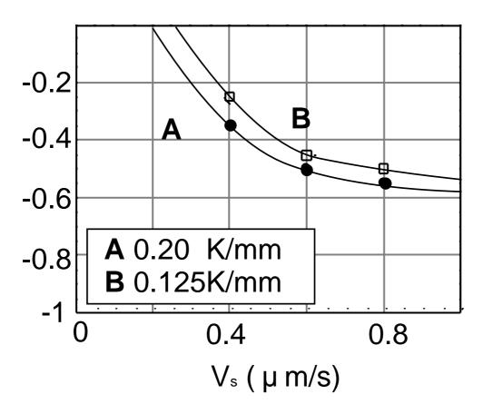
Fig. 26. Relationship between freezing rate and ice lens generation.
