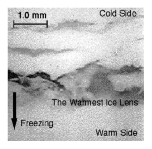
Fig. 15c. An image of the freezing sample 5s (water saturated non-uniform size glass particles) under the conditions of A0 ( $V_s = 0 \mu m/sec$ ,  $= 0.20 \, ^{\circ}C/mm$ ).
