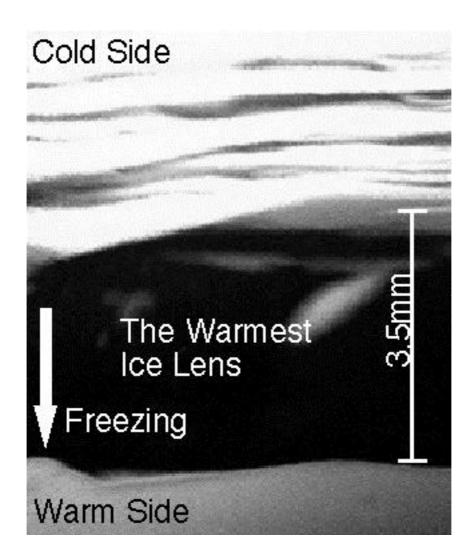
Fig. 15b. A image of the freezing sample 4 (glass particles) under the condition of D0  $(V_s=0~\mu\text{m/sec},~=0.33~^{\circ}\text{C/mm}).$
